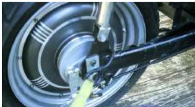
Place one strap on each side of the bike wrapped around the swing arm at the forward most position and angling forward at 45 degrees or more. This is to stop the bike from going backward. (shown here without cloth paint protection under hook merely for clarity)
