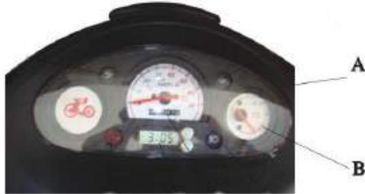
Power Meter – On the right side of the instrument panel (A) is a power gauge (B). Only when the needle is at the top of the arc is the bike charged for good road use. When it enters the broad band arc areas the bike is in danger of running out of power. When it reaches the bottom arc it will shut off to protect itself. A clock is in the center bottom and can be set by the two buttons to the right.
