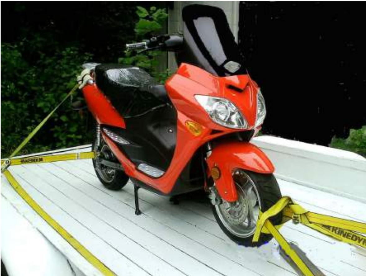
Place a second strap through the front wheel at the midpoint on the front (1/2 way up wheel) and pull this strap at a 45 degree angle toward the vehicle front to two tie down points
