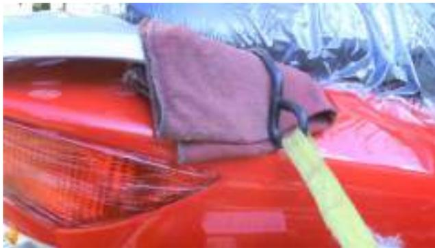
Place one strap on each side of the bike on the swing arm rear by the shock pulling backward at least 45 degrees or more. This is to prevent the bike from moving forward on braking of the transport vehicle.
