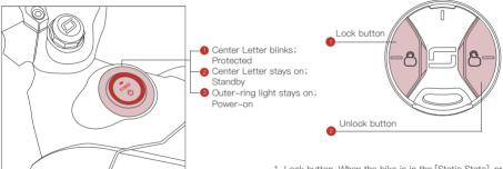
1. Lock button. When the bike is in the [Static State], press the lock button, and the start button flashes. The bike enters the [Locked State].
