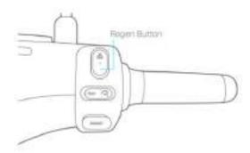
When you release throttle and let the Smartscooter® glide during riding, the regenerative braking function might be activated. It converts dynamic energy to electric energy, and puts the energy back into the Gogoro Network™ battery.
