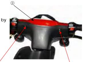
2. Remove master cylinder by removing the bolt ;
