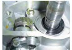
remove cylinder head and cylinder
