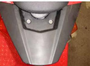
unlock oil pump cap and remove it, two tapping screw are exposed, remove them; remove tapping screw; then remove side cover
