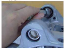
Install shock absorber bushing
