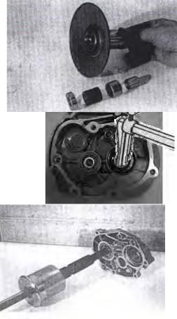
Remove left crankcase oil seal
