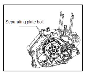
Use a special tool to screw off clutch locknut.
