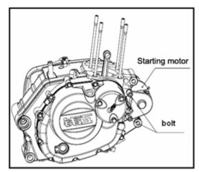
Screw off bolts on left front cover and left rear cover of crankcase.
