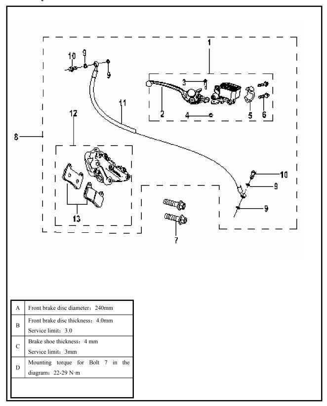
1 Oil pump block assembly 2 Hydraulic brake handle 3 Handle mounting bolt 4 Nut M6 5 Fixed cover 6 Bolt M6×23 7 Front hydraulic brake mounting bolt 8 Front hydraulic brake assembly 9 Washer 10 Oil hose mounting bolt 11 Brake hose assembly 12 Brake cylinder assembly 13 Brake shoe assembly
