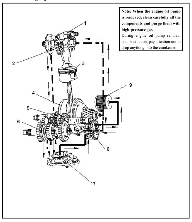
1 Rocker arm2 Cam mechanism3 Piston4 Crankshaft7 Filter screen8 Engine oil pump9 Filter element assembly
