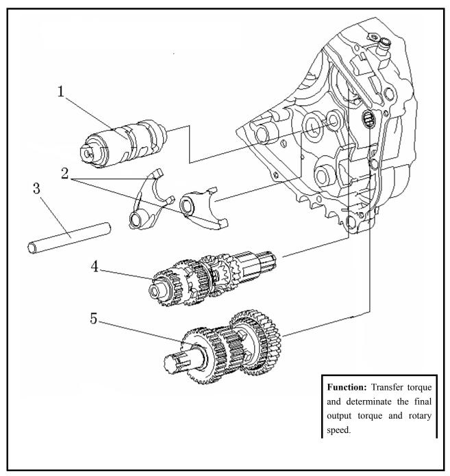
1 Gearshift drum 2 Shift fork 3 Shift fork shaft 4 Main shaft assembly 5 Countershaft assembly
