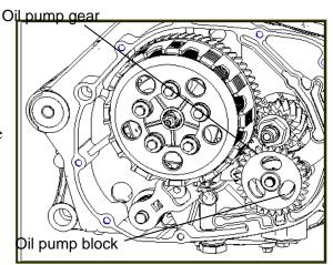
Screw off the screw Take down pump seat.
