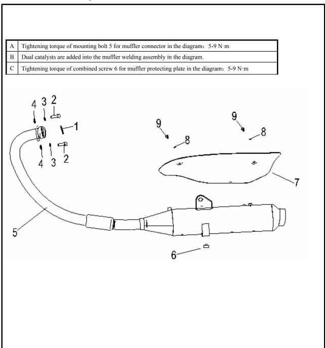
1 Exhaust pipe gasket assembly 2 Bolt M8×30 3 Washer 8 4 Spring washer 5 Muffler welding assembly 6 Muffler cushion rubber 7 Muffler decorative plate 8 Thermal insulation spacer 9 Combination screw
