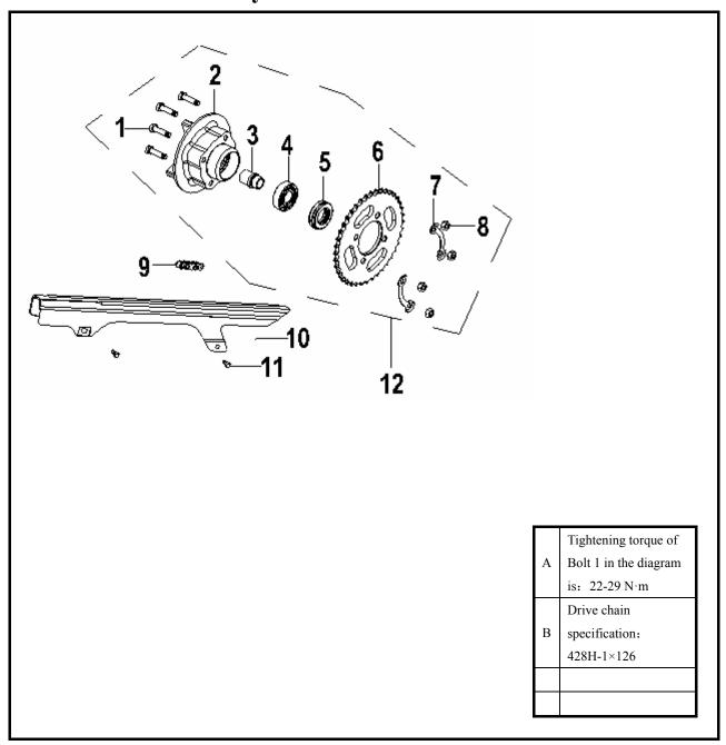
1 Sprocket mounting bolt 2 Sprocket hub 3 Chain drive sleeve 4 Rolling bearing 6204-2RS 5 Oil seal 6 Sprocket 43 teeth 7 Sprocket stopper 8 Nut M8 9 Chain 428H-1×126 10 Chain guard 11 Boss bolt
