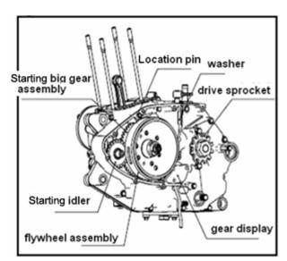
Use an electric or pneumatic tool to screw off flywheel locknut.
