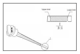
ruler into the engine. Do not tighten the ruler.
