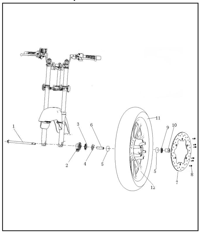
1 Front wheel shaft 2 Gear seat assembly 3 Gear seat oil seal 4 Drive plate 5 Bearing 6 Front wheel middle sleeve 7 Front brake disc 8 Front brake disc mounting bolt 9 Front wheel oil seal assembly 10 Front wheel left sleeve 11 Tubeless tyre 12 Front wheel rim
