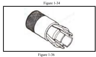
(2) Special tools for chassis overhaul: Front fork seal driver
