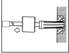
Lubricate front shaft, gear seat assembly, oil seal (lip), sleeve, bearing 6301-2RS, and middle sleeve.
