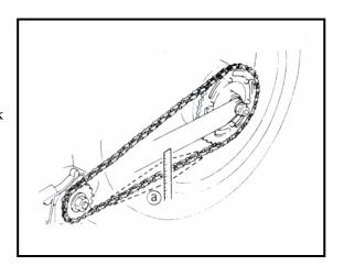
Screw off rear shaft nut and lock-nuts of adjusters on both drive chains.
