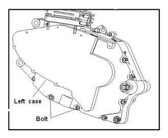
Remove left case block. Pull out shift fork shaft. Remove gearshift drum. Remove gearshift fork.
