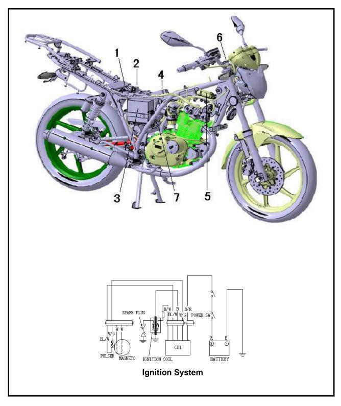
1 Relay 2 Scintillator 3 Battery 4 Igniter 5 High-voltage ignition coil
