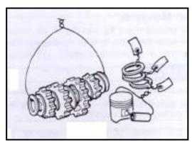
Pay special attention to the key fitting position before disassembly. The components that are not used any more shall be replaced on time before disassembly.
