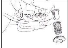
When the engine oil is completely drained, put back cleaned drain plug and sealing ring.
