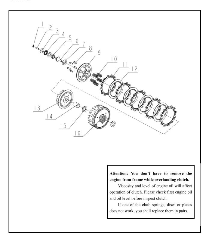
1 Nut 2 Cross recessed adjusting screw 3 Thrust washer 4 Plane needle bearing 5 Locknut 6 Bearing seat
