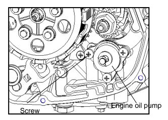
Remove the screw and take down pump cover. Disassemble oil pump
