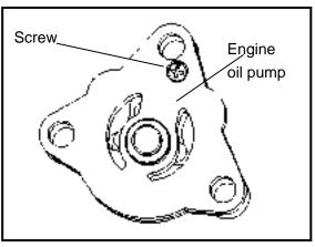
Check radial clearance between inner rotors Allowable limit: 0.2mm.
