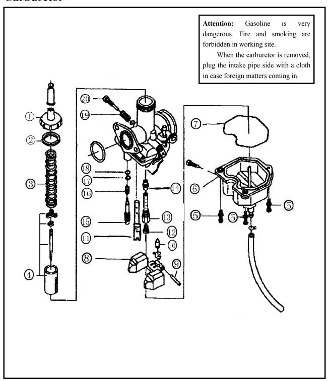
1- Upper cover 2- Upper cover seal ring 3- Plunger spring 4- Plunger assembly 5- Lower housing connecting screw 6- Lower housing assembly 7- Seal ring 8- Float assembly 9- Float pin 10- Needle valve core 11- Idle jet 12- Main jet 13- Main nozzle 14- Main foam pipe 15-Mixture screw 16- Mixture screw spring 17-Fixture screw washer 18- Mixture screw seal ring 19-Plunger adjusting screw spring 20- Plunger adjusting screw
