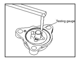
Check clearance between rotor end faces.
