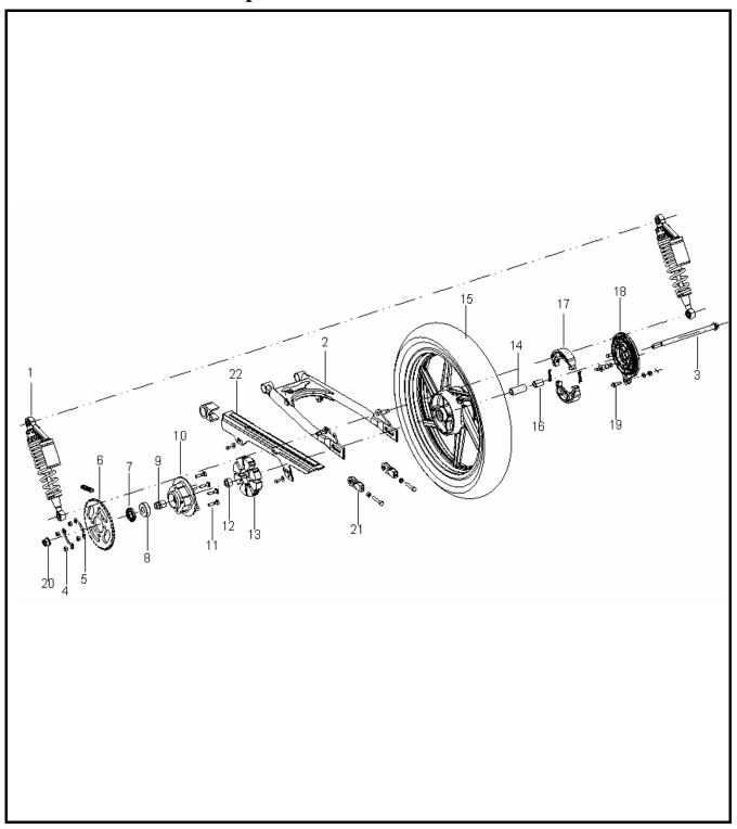
1 Rear shock absorber assembly 2 Rear brake rocker arm 3 Rear shaft 4 Nut M8 5 Sprocket stopper 6 Sprocket 43 teeth 7 Oil seal 8 Rolling bearing 6204-2RS 9 Chain drive sleeve 10 Sprocket hub 11 Sprocket mounting bolt 12 Rear wheel left sleeve assembly 13 Rear wheel buffer 14 Bearing spacer 15 Tubeless tyre 16 Rear wheel left sleeve 17 Rear braking shoe 18 Rear wheel hub 19 Bolt 20 Locking nut M14×1.5 21 Chain adjuster assembly 22 Chain guard
