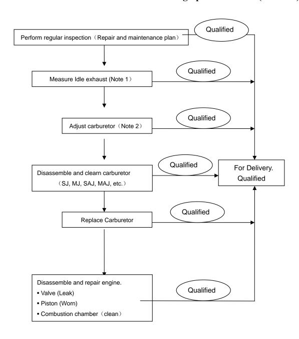
Note 1: Measure according to the idle speed measuring procedures.
