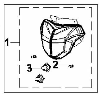
Avoid touching bulb glass with your bare hands during installation and staining it with oil, which may affect transparency, service life and luminous flux of bulb.
