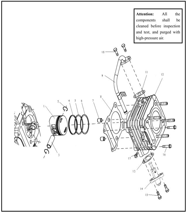
1 Piston 2 Retainer 3 Piston pin 4 Combined oil ring 5 Second compressing ring 6 Top ring 7 Location pin 8 Washer 9 Cylinder cover connecting bent pipe assembly 10 Bolt 11 Cylinder cover connecting bent pipe washer assembly 12 Cylinder block 13 Washer 14 Tensioner assembly 15 Bolt 16 Bolt 17 Screw
