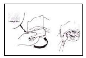
Installation of rubber hose (fuel, vacuum, or coolant): insert its end into bottom of connector so that there is enough room for the hose clamp to grip the connector. Install the rubber or plastic dust cover back to its originally designed position
