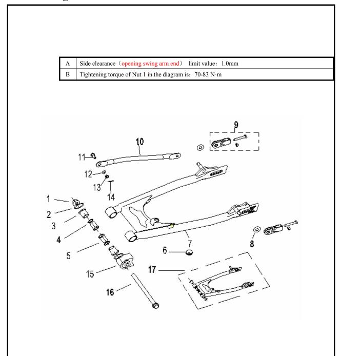
1 Locking nut M14X1.5 2 Dust ring assembly 3 Bush 4 Oil seal 5 Middle sleeve 6 Rubber gasket for protecting plate 7 Rear swing arm welding assembly 8 Washer φ12 9 Chain adjuster spacer 10 Connecting rod assembly 11 Bolt 12 Washer 13 Nut M8 14 Cotter pin 2×18 15 Chain protector 16 Rear swing arm bush 17 Rear swing arm assembly
