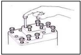
Fill lubricating grease into the groove during oil seal installation. Check if the oil seal is smooth and if there is any damage to it.
