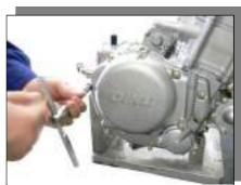
• Tighten Filter Cover plug to the specified tightening torque.
