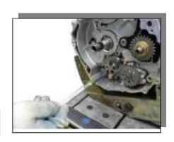
• Take out Special Tool; Oil Seal Guide, temporally fit Shift Pedal CP and make sure gear is shifted properly. Also make sure reverse locking operation.
