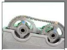
Apply oil to Camshafts attaching portion, and install
