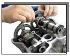
• Apply oil to Cam Support and install in position.
