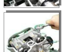
Depress Chain Tensioner plunger into the bottom position by Special Tool; Chain Tensioner Tool and then Install Tensioner.
