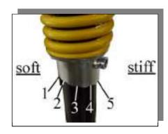
●Turn the adjusting sleeve on front shock absorber to the desired position with the wrench.
