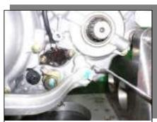
Apply grease onto front and rear surfaces of Sprocket 14T, and install it in position.
