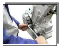
★ Make sure again the tightening torque of Primary Gear fixing nut.
