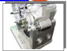
• Apply TB #1344 to Reverse Arm Lever threads (M6), and install along with Reverse Arm Spring.
