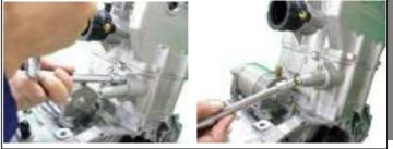
Adjust valve clearance with thickness gauge adopted at TDC position in the following procedures;
