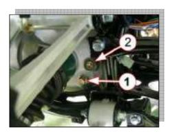
• Tighten the oil level plug [1] and oil filter plug [2] to the specified torque.
