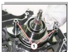
• Remove the crank balance shafts [1].
