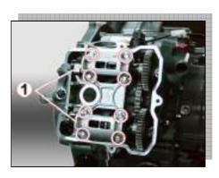
• Remove the pins and camshafts.
