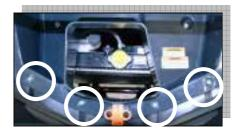
• Remove headlight by unscrewing the screws [C]×6
