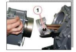
• Remove the piston by removing the piston pin circlip [1].
