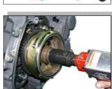
• Install the special tool to the crankshaft end.
