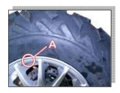
• If the tire is removed, inspect the air sealing surfaces [A] of the rim for scratches or nicks. Smooth the sealing surfaces with fine emery cloth if necessary
