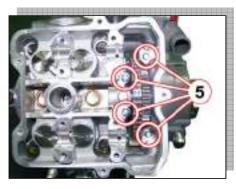
• Remove the cylinder head bolts (M10) and washers.
