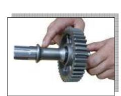
• Install the bearing with the special tool.
