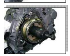
• Remove the generator rotor with the special tool.
