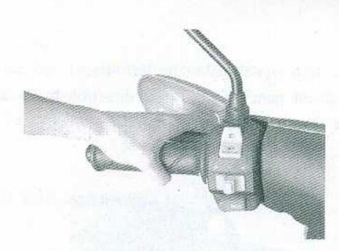
Turn on main switch and press down horn switch button to sound horn.
