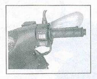
Press down starter switch button to use electric starter.
