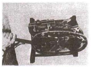
26. Removing the sprocket on the crankshaft
