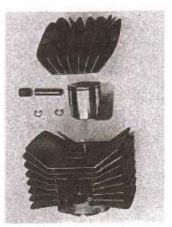
3. Cylinder piston, Cylinder head
