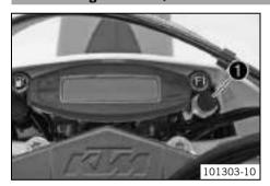
The light switch **1** is on the right of the speedometer.
