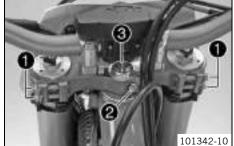
Loosen screws 1. Remove screw 2. Loosen and retighten screw 3.
