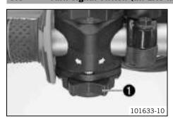
Turn signal switch • is fitted on the left side of the handlebar.
