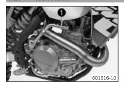
The kick starter **1** is fitted on the right of the engine.
