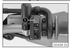
The emergency OFF switch  $\ensuremath{f 0}$  is fitted on the right side of the handlebar.
