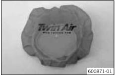
Fit a sand cover on the air filter.
