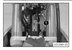
The type label • is fixed to the front of the steering head.
