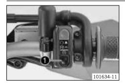
The electric starter button **1** is fitted on the right side of the handlebar.
