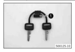
The key number • for the steering lock is stamped onto the key connector.
