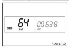
Press the button priefly and repeatedly until SPEED appears on the left side of the display.
