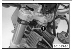
Steering lock • is fitted on the left side of the steering head.
