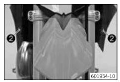
Mount and tighten screws ②.
