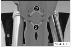
Position the front fender. Mount and tighten screws ②.
