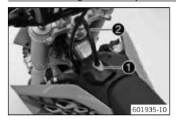
Replace the filler cap and turn clockwise until the release button ● locks in place.
