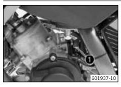
Choke lever **1** is fitted on the left side of the carburetor.
