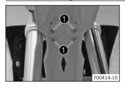
Remove screws ①. Remove the front fender.
