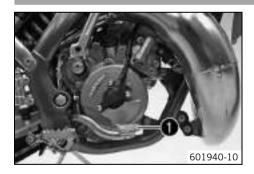
Foot brake lever **1** is located in front of the right footrest. The foot brake lever is used to activate the rear brake.
