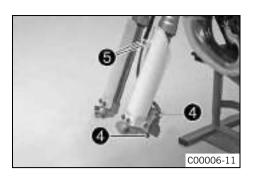
Position brake caliper, mount and tighten screws 4. Guideline
