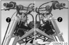
Mount and tighten screws **7**.
