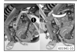
The kickstarter **1** is fitted on the right of the engine. The kickstarter can be swiveled.
