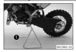
The fixture for the plug-in stand • is located on the frame on the left side of the vehicle
