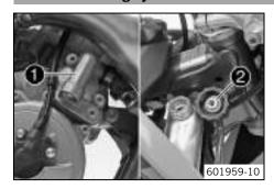
The water pump **1** in the engine forces the coolant to flow.
