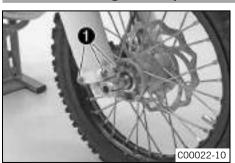
Position the fork protection on the right fork leg. Mount and tighten screws ①.
