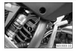
The shock absorber part number lacktriangle is stamped on the top of the shock absorber above the adjusting ring on the engine side.
