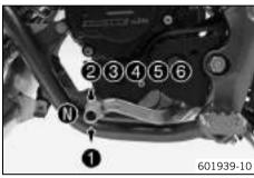
The gear positions can be seen in the photograph. The neutral or idle position  $\mathbf{0}$  is between the first and second gears.
