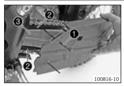
Position the chain guard. Mount cable binder •.
