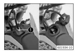
Press release button ●, turn the filler cap counterclockwise, and lift it free.
