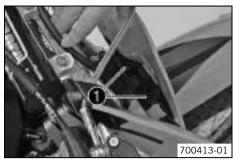
Position the start number plate with the drill holes onto the holding lugs • of the fender.
