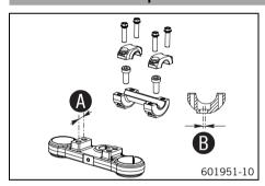
On the upper triple clamp, there are 2 holes at a distance of **4** to each other.
