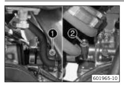
The idle setting of the carburetor has a big influence on the starting behavior, stable idling and the response to throttle opening. That means that an engine with a correctly set idle speed is easier to start than if the idle is set wrongly.
