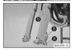
Position brake caliper, mount and tighten screws 8.
