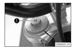
Turn adjusting screw 1 clockwise all the way.
