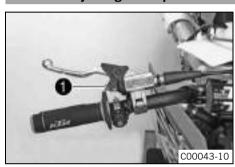
Adjust the basic position of the clutch lever to the size of the rider's hand using adjusting screw ●.
