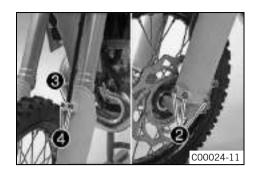
Position the fork protection on the left fork leg. Mount and tighten screws 2.
