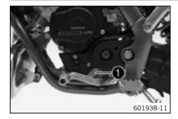
The engine number • is stamped on the left side of the engine under the engine sprocket.
