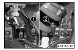
Screw in idle air adjusting screw 2 all the way and turn it to the specified basic position.
