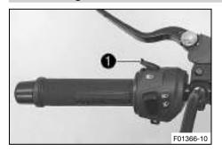
The high beam flasher button **1** is fitted on the left side of the handlebar.
