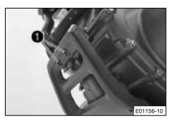
Position engine guard. Mount screws 1 but do not tighten yet.
