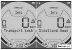
**Transport Lock** appears on the display if transport mode is activated.
