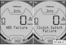
ABS Failure appears on the display if the ABS is no longer active.
