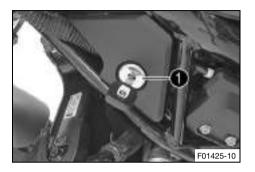
The seat lock **1** is located at the front left below the fuel tank. The seat lock can be unlocked using the ignition key.
