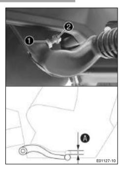
Release nut 1 and use screw 2 to adjust the specified free travel 1.
