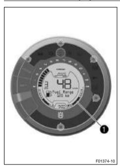
The fuel tank contents are shown in area of the display. The fuel level indicator consists of bars. The more bars are lit, the more fuel is in the fuel tank.
