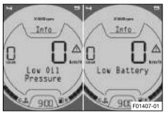
**Low Oil Pressure** appears on the display if the oil pressure is too low.
