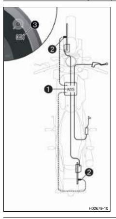
The ABS module ①, which consists of a hydraulic unit, ABS control unit, and return pump, is installed under the fuel tank.
