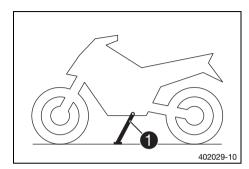
Side stand **1** is located on the left of the vehicle. The side stand is used for parking the motorcycle.
