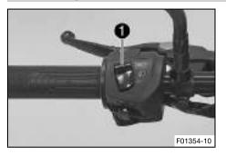
Light switch is fitted on the left side of the handlebar.
