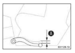
Move the foot brake lever back and forth between the end stop and the contact to the foot brake cylinder piston and check free travel .
