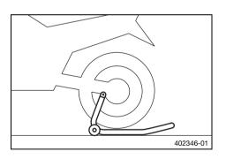
Mount the supports of the lifting gear.
