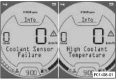
**Coolant Sensor Failure** appears on the display if the coolant temperature sensor is faulty.
