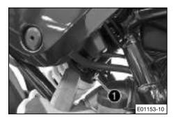
Set the spring preload by turning adjusting ring using the hook wrench and the extension from the tool set.
