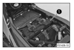
The tool set 1 is located under the seat.
