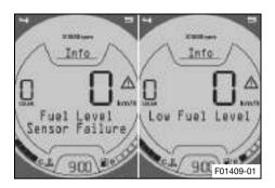
Fuel Level Sensor Failure appears on the display if the fuel level indicator is faulty.
