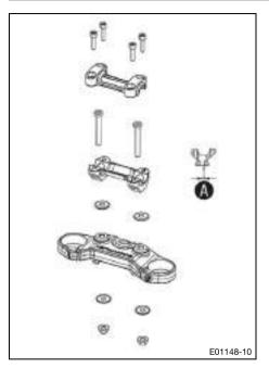
The holes on the handlebar support are placed at a distance of **A** from the center.
