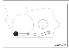
Shift lever **1** is mounted on the left of the engine.
