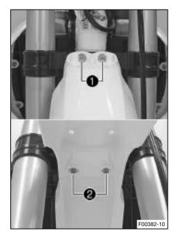
11.17 Installing front fender
