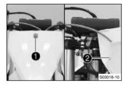
Remove screw 1. Swivel the start number plate to one side. Remove screw **2** and take off the brake line guide and start \_ number plate.
