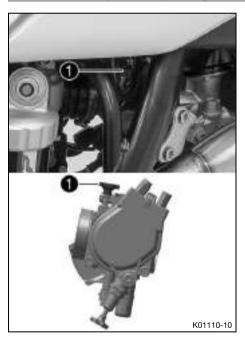
The idle setting of the throttle valve body substantially influences the vehicle's starting behavior, a stable idle speed, and the vehicle's response when the throttle is opened.
