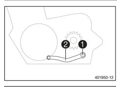
Remove screw **1** with the washers and take off shift lever **2**.
