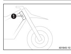
The vehicle identification number ① is stamped on the right side of the steering head.
