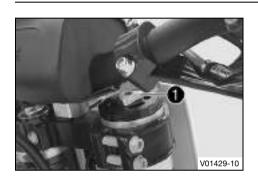
Turn adjusting screw 1 clockwise all the way.
