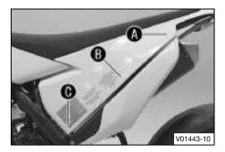
Pull off the air filter box cover sideways in areas (A), (B) and (C) and take off toward the rear.
