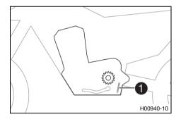
The engine number **1** is stamped on the left side of the engine.
