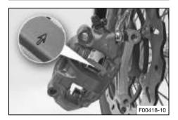
Clean the brake caliper and spring plate.Ensure that the spring plate is correctly positioned.
