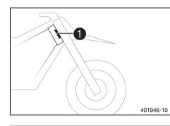
The type label 1 is fixed to the front of the steering head.
