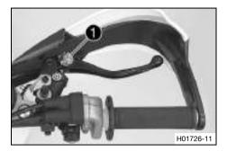
Adjust the basic position of the hand brake lever to your hand size by turning adjusting wheel ①.
