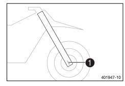
The fork part number **1** is stamped on the inside of the axle clamp.
