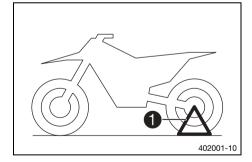
The support for plug-in stand **1** is the left side of the wheel spindle.
