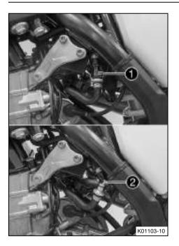
Clean plug-in connection ① of the fuel line thoroughly with compressed air.
