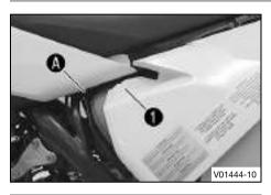
Attach catch 1 of the air filter box in area A and push forward.
