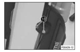
Position the brake line and the clamp. Mount and tighten screws **1**.
