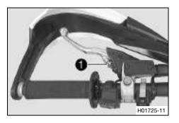
Adjust the basic position of the clutch lever to your hand size by turning adjusting screw **①**.
