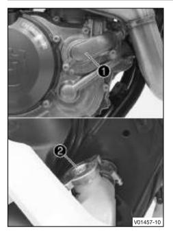
Water pump 1 in the engine circulates the coolant.
