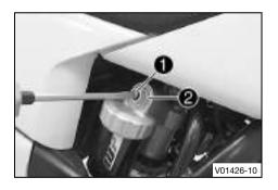
Turn adjusting screw ① clockwise with a screwdriver as far as the last perceptible click.
