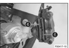
Press the brake piston back into the basic position and ensure that brake fluid does not flow out of the brake fluid reservoir; extract some if necessary.
