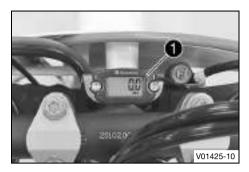
The service hour counter ① is fitted in front of the handlebar. It shows the total number of service hours of the engine. The service hour counter begins counting when the engine is started and stops when the engine is switched off.
