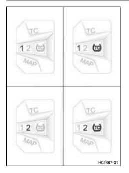
The combination switch is fitted on the left side of the handlebar. **Possible states**
