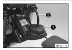
Mount fuel tank filler cap **1** and turn it clockwise until the fuel tank is tightly closed.
