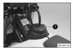
Turn fuel tank filler cap lacksquare counterclockwise and lift it off.
