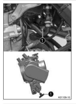
Cold start button **1** is fitted to the bottom of the throttle valve body.
