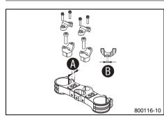
On the upper triple clamp, there are 2 holes at a distance of A to each other.
