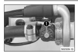
Electric starter button 1 is fitted on the right side of the handle-
