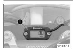
The run hour counter ① is fitted in front of the handlebar. It shows the total number of service hours of the engine. The service hour counter begins counting when the engine is started and stops when the engine is switched off.
