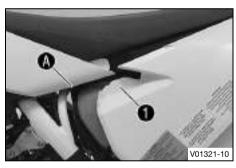
Attach catch 1 of the air filter box in area 1 and push forward.
