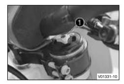
Turn adjusting screw clockwise all the way.
