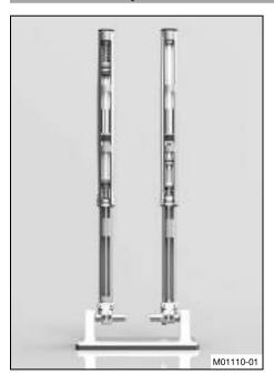
Air suspension **WP Suspension AER 48** is used in the fork. In this system, suspension is located in the left fork leg and damping in the right fork leg.
