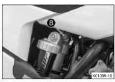
Hold the shock absorber and remove screw 8.
