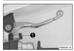
Adjust the basic position of the hand brake lever to your hand size by turning adjusting screw 1.
