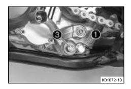
Mount and tighten screw plug with the O-ring. Guideline
