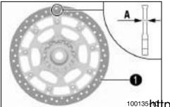
Check the thickness of the front and rear brake discs at multiple points on each brake disc to ensure it is at least thickness .
