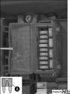
Remove the defective fuse.
