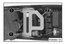
Position retaining bracket 2 and mount and tighten screws 1.
