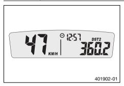
Press one of the buttons until DST2 appears on the speedometer.
