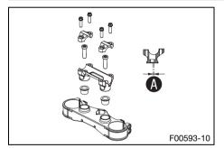
The holes on the handlebar support are placed at a distance of  $oldsymbol{A}$  from the center.
