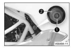
Turn adjusting screw 1 all the way clockwise with a socket wrench.
