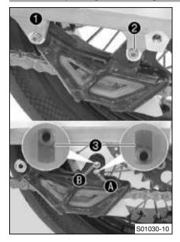
Remove screws 1 and 2. Take off the chain guide.
