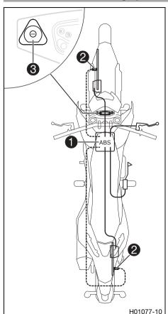
The <u>ABS</u> unit **1**, which consists of a hydraulic unit, ABS control unit, and return pump, is installed under the seat. One wheel speed sensor **2** is located in each case on the front and the rear wheel.
