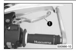
The hand break lever is fitted on the right side of the handlebar. The hand brake lever operates the front brake.
