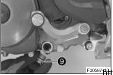
Mount and tighten screw plug
