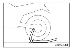
Insert the adapter into the rear wheel stand and screw into the swingarm on both sides.
