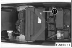
Position the engine electronics control unit 11.
