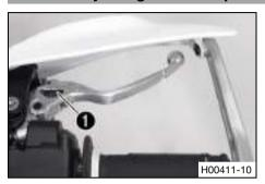
Adjust the basic position of the hand brake lever to your hand size by turning adjusting wheel 1.
