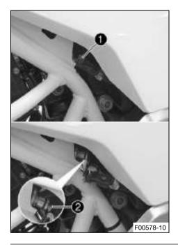
Clean plug-in connection 1 of the fuel line thoroughly with compressed air.
