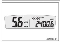
Press one of the buttons until AVG, ART and ODO appear in the speedometer.
