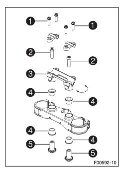
Remove screws 1. Take off the handlebar clamps. Remove the handlebar and lay it to one side.
