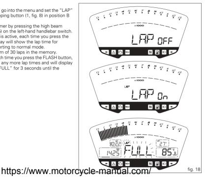
When you switch the LAP function off using the menu. the lap in progress is not saved.
