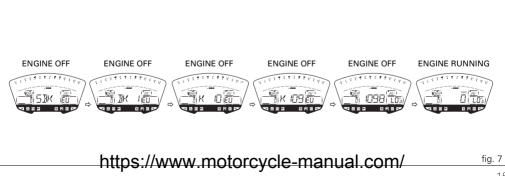
At Key-On, the instrument panel always shows the following information (de-activating any previously activated functions):
