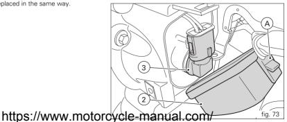
Notes It is not necessary to disconnect the main wiring loom cable in order to replace the headlight bulbs.
