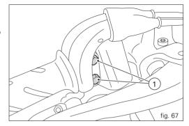
Adjustment of the throttle cable free play In all handlebar positions, the throttle twistgrip should have free play of 1.5 - 2.0 mm measured at the edge of the twistgrip. If necessary, adjust using the adjusters (1 and 2, fig. 69) located on the steering tube on the right-hand side of the motorcycle.
