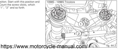
The STANDARD factory settings are as follows: compression: 3/4 turns (1098), 8 clicks (1098S - 1098S Tricolore); rebound: 12 clicks (1098), 10 clicks (1098) - 1098S Tricolore); Spring preload (1098)(A, fig. 44.1): 18 mm; corresponds to an actual preload of 9 mm. Spring preload (1098S - 1098S Tricolore); starting with the adjuster screwed FULLY OUT, screw it in clockwise 8 turns; corresponds to an actual preload of 8 mm.
