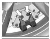
Brake-pad wear limit of T parking brake
