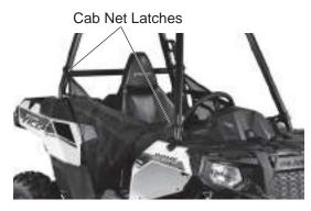
Always inspect cab nets and latches for tightness, wear and damage before each use of the vehicle. Use the strap adjusters to tighten any loose straps. Promptly replace worn or damaged cab nets and latches with new cab nets and latches. Please see your authorized POLARIS dealer.
