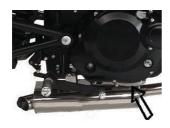
4. Tighten the oil drain plug and fill it with fresh engine oil, pour 1400 ml into the oil filler, before gently tightening the filler cap.
