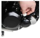
3. Remove the drain plug from the strainer cover on the engine bottom to drain the oil.
