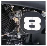
To help starting, the vehicle is equipped with a carburetor enrichment system: Plunger carburetor: To start a cold engine, raise the enrichment lever to the highest position. After starting, lower the lever to half way and
