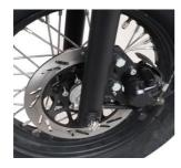
It is essential to check the front and rear brake rotors to make sure they are not below the minimum thickness. If wear exceeds the mark, the brake rotor and pads shall be replaced with new ones.
