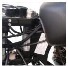
Chassis number (or VIN code) is on the steering stem frame tube. Engine number is on the lower left side of the crankcase. Metal nameplate is on the riser pipe of chassis, showing the main technical parameters, manufacturer and date of production of the motorcycle.
