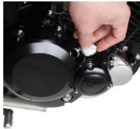
3. Remove the drain plug from the strainer cover on the engine bottom to drain the oil.
