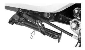
Side stand can be operated by sitting on vehicle with your left foot by pushing it away from the vehicle till it stops.
