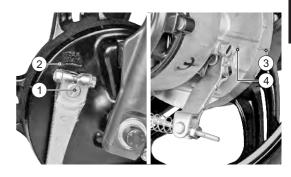
When the brake is applied, wear limit index mark (1) on the front brake cam should be within the wear limit indicator (2) on the front brake panel.
