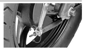
4. Turn the adjuster nut in clockwise direction for reducing the free play or in anti-clockwise direction for increasing the free play.
