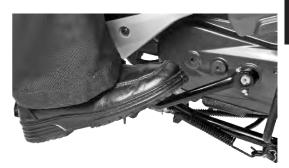
Keep your foot on the lever extension as shown in the figure. Kick the lever from top and stroke to bottom with rapid motion.
