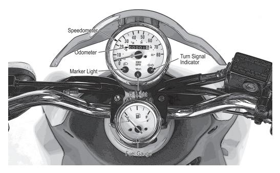
**Speedometer -** Indicates the speed in both km/hour and MPH. Mileage Counter - The total mileage traveled in kilometers is indicated by the first five digits (white writing on black background). The last digit indicates 1/10th of a kilometer (100 meters). To convert from kilometers to miles, multiply this number by .625.
