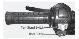
Move the switch to the right to activate the right turn indicator. Move the switch to the left to activate the left turn indicator. Press the white button in the middle to turn off the turn indicator.
