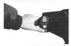
Turn on main switch and press down horn switch button to sound horn.
