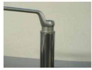
• Tighten cap to the specified torque.
