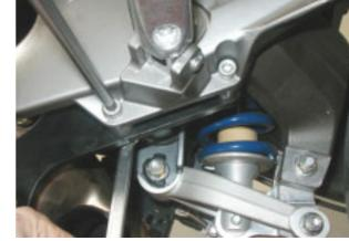
Move the left footrest plate and release the gear shift transmission. Remove the left footrest plate.
