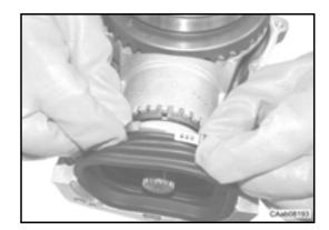
Lock the clamp (12) with suitable pliers.
