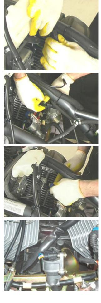
• Connect the connector on the end of the throttle position sensor.
