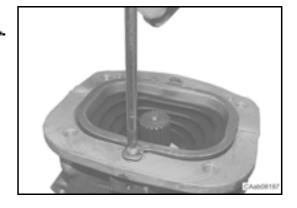
Assemble the plug (**3**) and the washer (**2**). Tighten the plug to the prescribed torque.
