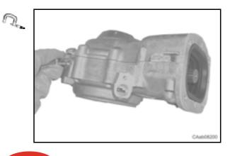
Assemble the breather (6) and the washer (5). Tighten the breather (6) to the prescribed torque.
