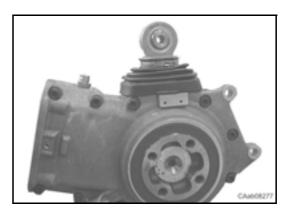
Remove the clamps (9) and (11). Remove the boot (14).
