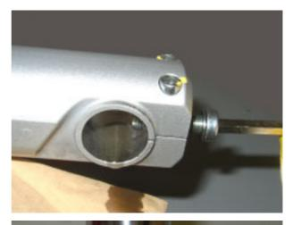
Remove the dust seal, pry with a screwdriver.
