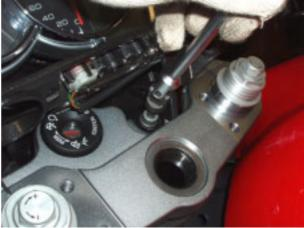
Working on either side, remove the screw securing the headlight subframe to the bottom yoke.
