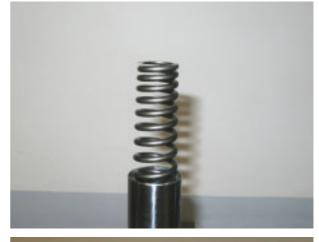
• Start the plug onto stanchion tube, pay attention not to damage O-ring.
