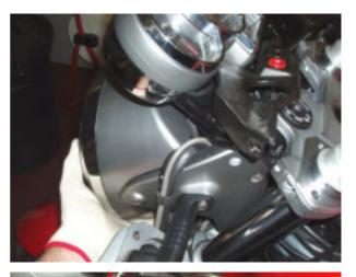
• Working on either side, remove the screw securing the fork legs to the steering head.
