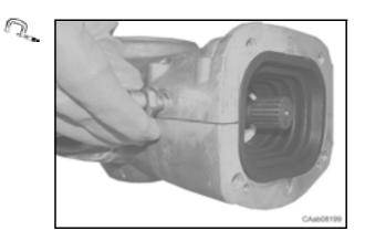
Fill the transmission with the prescribed oil. Assemble the plug (**3**) and the washer (**2**). Tighten the plug to the prescribed torque.
