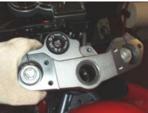
• Bend the safety washer onto steering tube.
