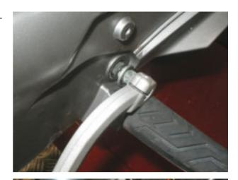
• Loosen and remove the two upper screws.
