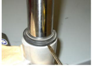
Pull up the dust seal to remove it.
