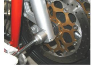
• Tighten the wheel shaft clamp screws to the specified torque.
