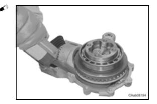
Assemble a new seal ring (1) using the special tool. Lubricate the seal ring (1).
