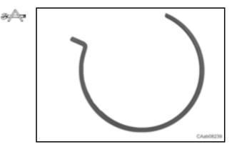
Warning: the locking ring (1) must be pushed in its seat.
