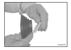
Assemble the boot (14) to the support (8). Assemble the clamp (12).
