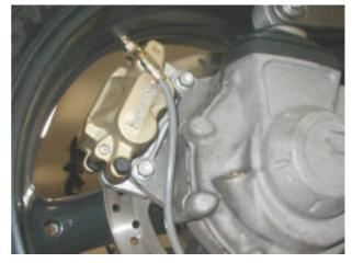
• Loosen and remove the four screws of the rear brake hose guides.
