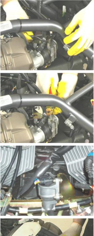
• Disconnect the stepper motor connector.
