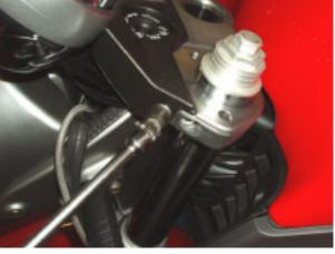
• Slide out the steering head, moving it toward the instrument panel.
