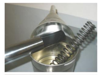
**NOTE** Push the rod inside the sleeve so that oil will flow out more easily.
