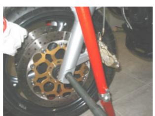
• Tighten the clamp screws (nut side) to lock the wheel shaft.
