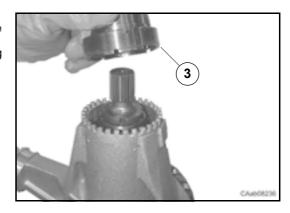
Assemble the seal ring (3) to the ring nut (2) with the special tool and a hammer.
