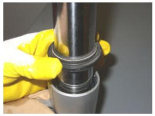
Remove the snap ring from inside the sleeve using a screwdriver.
