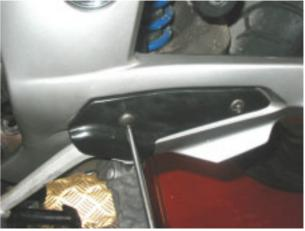
• Loosen the gear shift lever screw.
