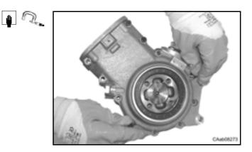
Assemble the ring (15) to the housing.
