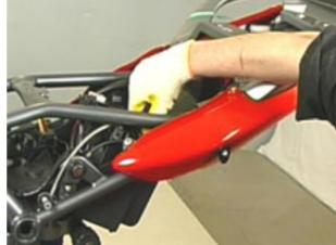
Fit the clutch bleed hose.Fill the clutch system with fluid.
