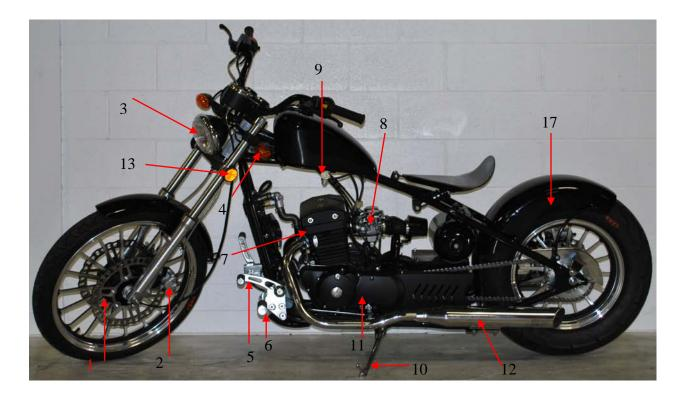
Front rotor (left) 2. Front brake caliper (left) 3. Front Headlight 4. Front left turn signal 5. Gearshift lever 6. Foot peg 7. Engine 8. Choke valve 9. Petcock 10. Kickstand 11. Engine serial number 12. Left side exhaust signal 13. Front Reflector
