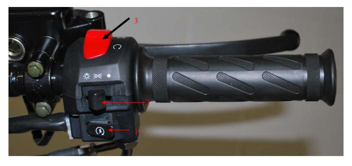
1.Electric start button 2. Headlight switch 3.Engine cut-off switch
