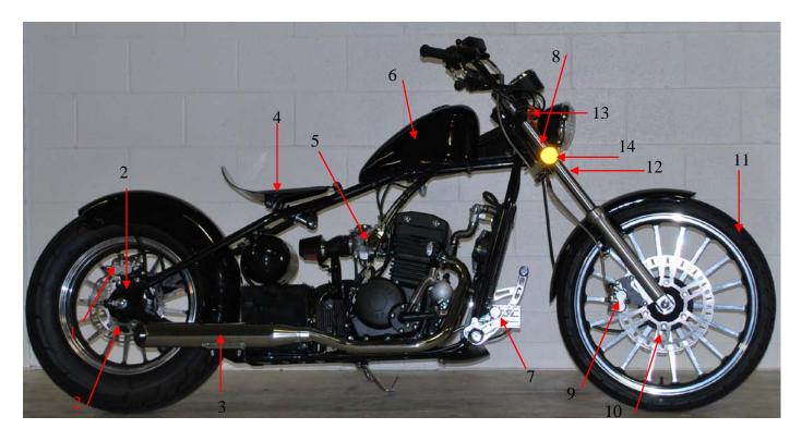
Rear brake caliper 2. Rear rotor 3. Right side exhaust 4. Seat 5. Carburator
