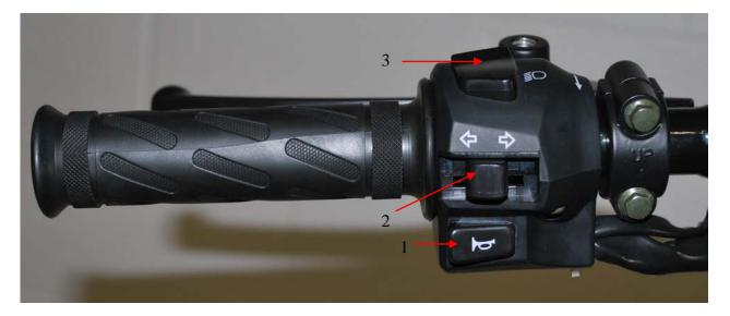
Horn button 2. Turn signal switch
