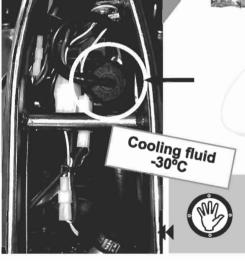
When filling the radiator, use cooling fluid designed for lightweight alloy motors.
