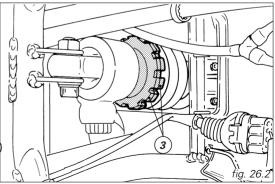
The Öhlins shock absorber features also length adjustment. It allows to adjust the seat height regardless the spring preload.
