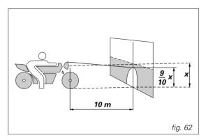
**The height of the light beam** can be corrected using the screw (1, fig. 63) on the left side of the headlamp. Turn the screw clockwise to lower the beam, anticlockwise to raise it.
