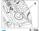
A: Oil Filler Location B: Oil Level Indicator C: Upper Level D: Lower Level Engine Oil: Check engine oil level daily.
