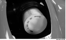
Clean dust and debris from the air filter housing; then remove the cotton-fabric safety element using care not to allow dirt and debris to enter the engine.
