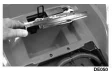
The storage compartment is located beneath the tool storage tray. Remove the tool storage tray to access the storage compartment.
