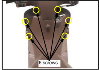
Remove the  $1 \times 2$  mounting screws of front spoiler from the inner box.
