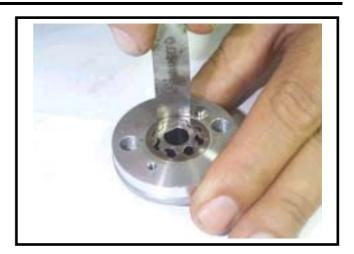
Check clearance between inner and outer rotors.
