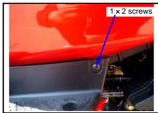
Remove the 1 mounting screw between the body cover and front center cover.
