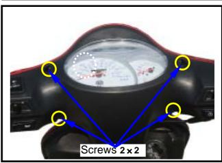
Remove the headlight connector. Remove the front handle cover.
