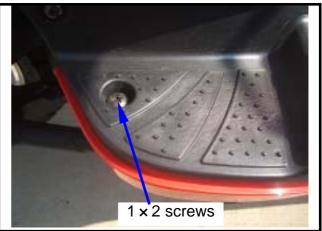
Remove the  $1 \times 2$  mounting screws between the left/right side cover and the frame.
