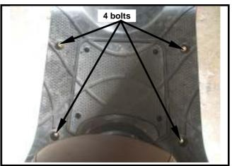
Remove the 4 screws from the battery cover.
