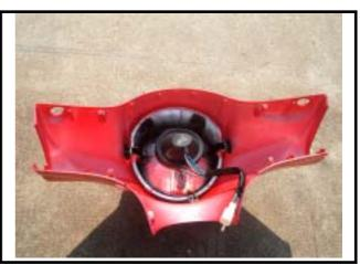
Remove the mounting screws (2 screws) between the rear handle cover and the frame.
