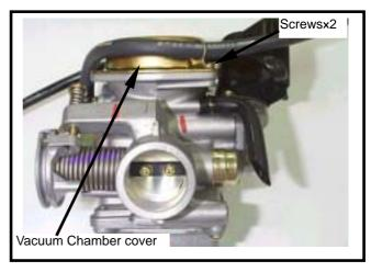
Remove compress spring and vacuum piston.
