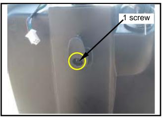
Remove the screw on the main switch. Remove the main switch cover.
