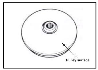
Install siding pulley assembly onto crankshaft.
