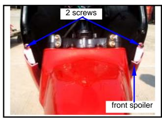
Remove the screw on the front inner box.
