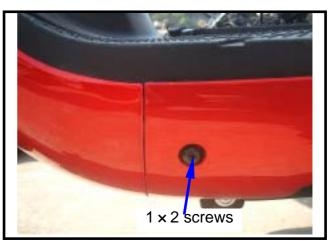
Remove the  $2 \times 2$  mounting bolts between the under cover and the frame.
