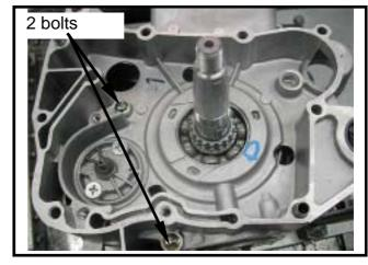
Install the cam chain tensioner.
