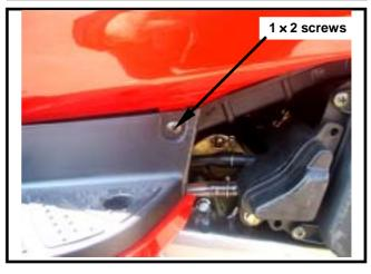
Remove the  $1 \times 2$  screws between the left/right side cover and the floor panel.
