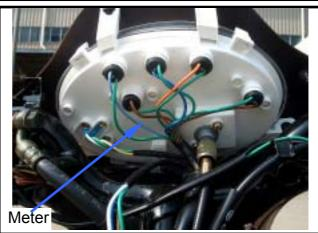
Remove the speedometer cable.
