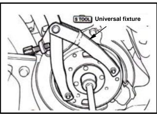
Install the cooling fan. (4 bolts)
