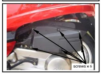
Remove the air cleaner element (2 screws). With compressed air to clean dirty around the element. Replace it if it is too dirty to clean.
