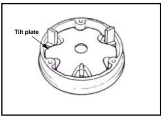
Remove weight rollers from sliding pulley.
