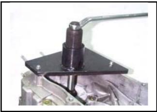
Remove the crankshaft from the right crankcase.
