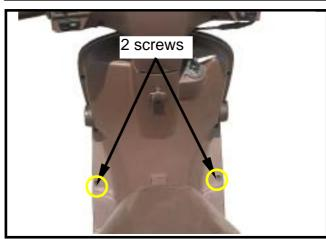
Remove the  $1 \times 2$  mounting screws of front spoiler from the inner box.
