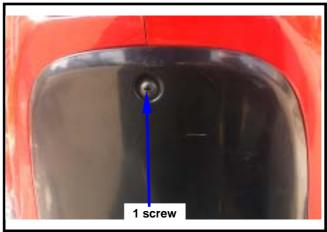
Remove the  $1 \times 2$  screws between the body cover and the floor panel.
