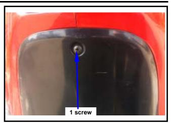
Remove the 4 screws from the battery cover. Remove the the battery cover. Remove the front center cover.
