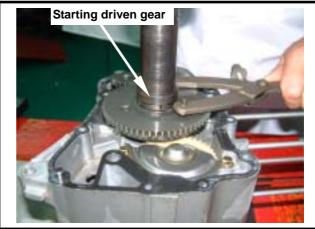
Remove starting clutch, starting reduction gear, and shaft.
