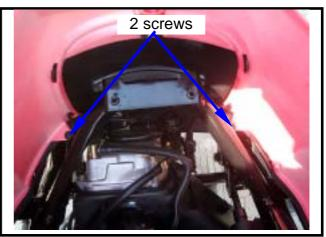
Remove the  $2 \times 2$  mounting screws between the body cover and the rear fender.
