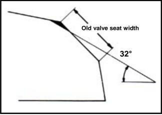
Use 60° cutter to cut a quarter lower part out. Remove the cutter and check new valve seat.
