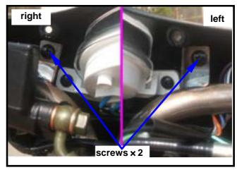
Remove the speedometer cable.
