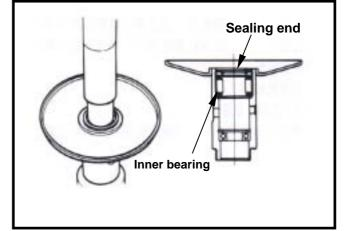
Install a new inner bearing.
