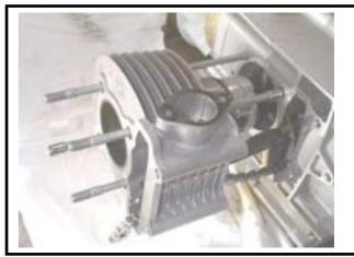
Remove cylinder gasket and lock pins
