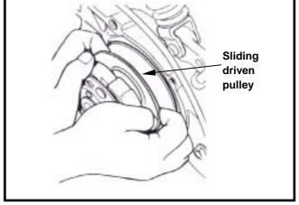
Install the clutch set with driving belt onto the driving shaft.
