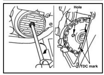
Remove camshaft holder nut and washer.
