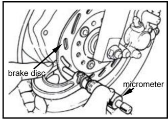
Remove the brake disc from wheel. Check the disc for deformation and bend.
