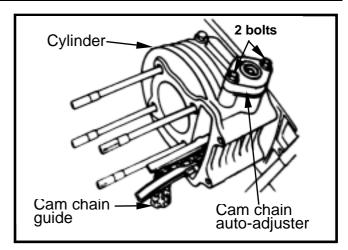
Remove cam chain plate. Remove cylinder.
