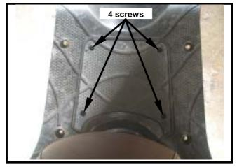
Remove the front center cover mounting screw.
