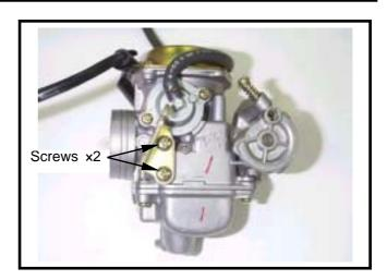
Remove the screws (screw x 2) of the air cut-off valve and its cover.
