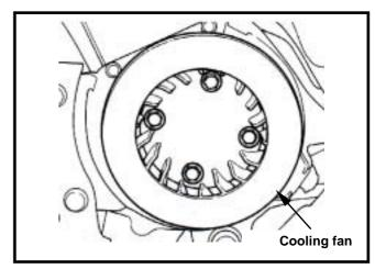
Install the cooling fan shroud. (4 bolts)
