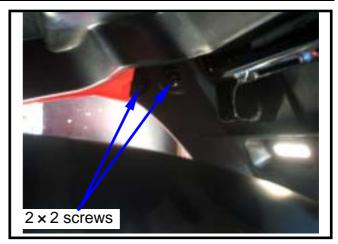
Remove the  $1 \times 2$  mounting screws between the body cover and the floor panel.
