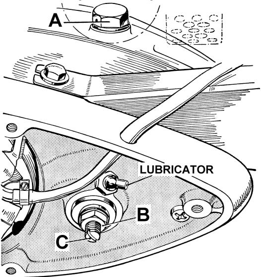
Fig. 7. Clutch control adjustment, with outer cover removed.
