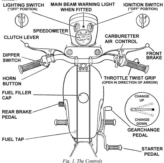
The lower illustration shows the controls for the Bantam Supreme.
