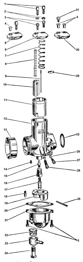
Fig. 5. The Amal concentric carburetter
