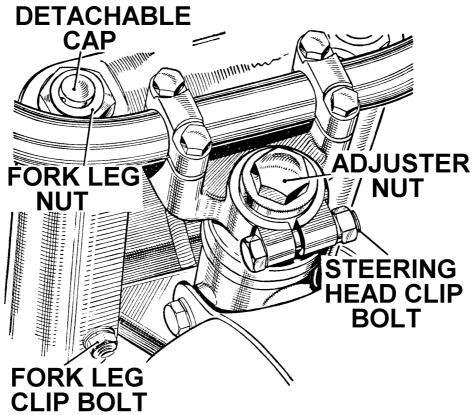
Fig. 9. Front fork and steering head (Bantam Supreme)
