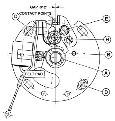
Fig. 2. The Contact Breaker
