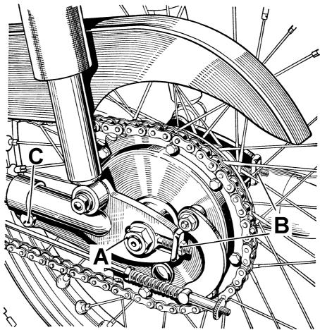
Fig. 8. Rear Chain Adjustment
