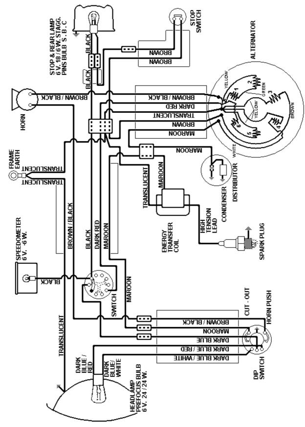
Fig. 11. Wiring Diagram (Bushman model)
