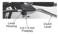
**Tip:** The starter interlock switch is dependent on the clutch lever freeplay being set correctly to ensure activation of the clutch safety switch.
