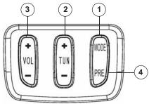
**Mode Button**: Press and hold the MODE button until the system enters the audio system mode menus. Then press and release the MODE button until the desired mode menu displays.
