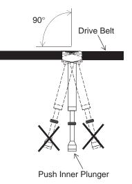
10. To calculate belt tension (deflection) subtract the smaller measurement from the larger measurement and record it.
