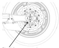
Check for movement in wheel bearing area
